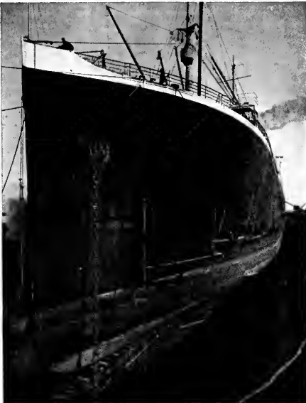
The steamer "Minnesota" in Hunter's Point dry dock being coated with composition furnished by the American Marine Paint Company of San Francisco.
